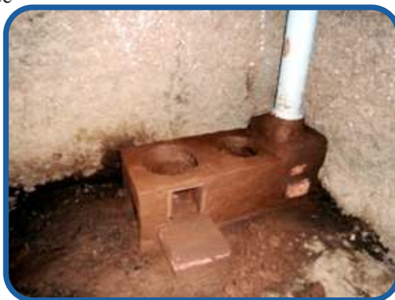
Freshly constructed Sarala stove
